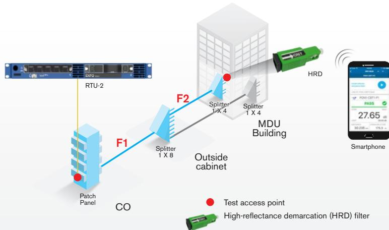
Figure 2. Link certification in a PON architecture with end-to-end connectivity.
