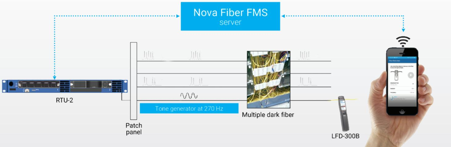
Figure 3. Source/tone mode for fibre identification.
